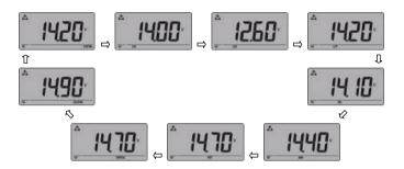
Press the **SET UP button** again, the selected battery type will be solid On and confirmed.
